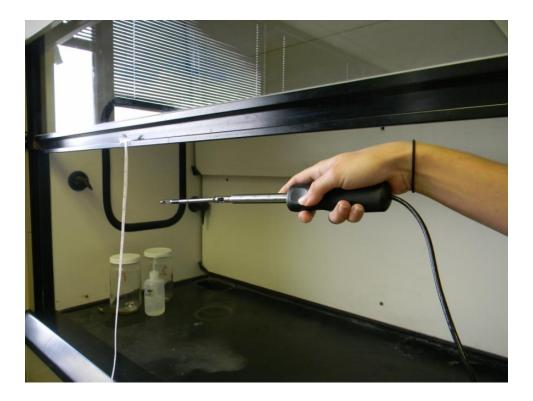
6. Repeat steps 1-5 for each air flow face velocity test.
