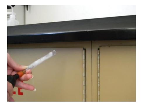
3. Continuously discharge smoke under the bottom air foil.
